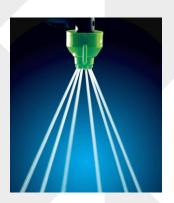
Six solid liquid streams in a pattern designed to optimise fertiliser distribution. For optimum placement and minimum crop scorch set the boom height at 50 cm above crop.
